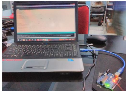
Gambar 9. Proses *upload sketch* ke arduino
